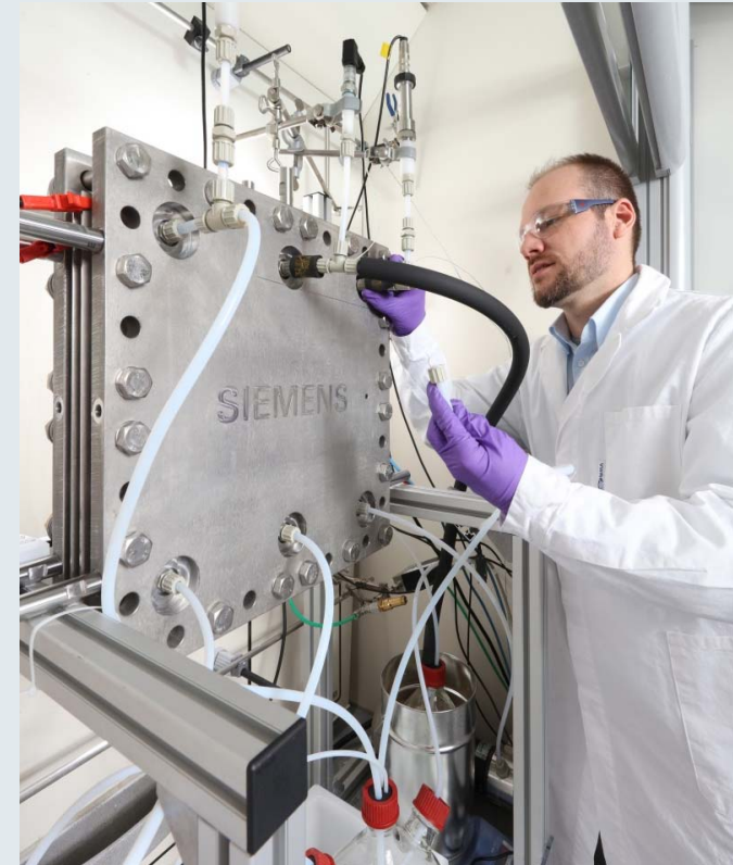
First test operation of the 300 cm 2 electrolysis cell at Siemens AG
